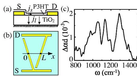
FIG. 1. (Color online) (a) FET schematics. (b) A sketch of the V-shaped electrodes between which the IR scans were taken. (c) The voltage-induced absorption spectrum  $\delta ad$  of one of the FET devices studied. The sharp absorption peaks are the IR-active vibrational modes of P3HT.
