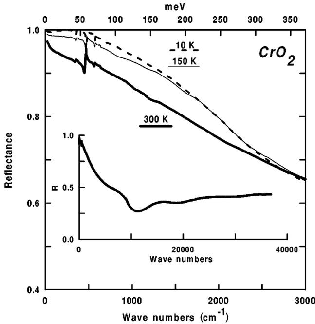
FIG. 1. Reflectance of  $\text{CrO}_2$  at 10 K, 150 K, and 300 K. Far-infrared reflectance is strongly temperature dependent and increases by as much as 7% at  $500 \text{ cm}^{-1}$ . The inset shows the 300 K reflectance over a broader energy scale.
