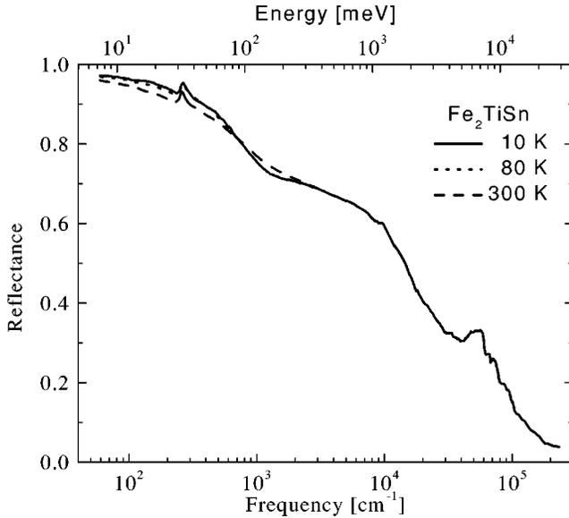
FIG. 1. The reflectance data of  $\text{Fe}_2\text{TiSn}$  at 10, 80, and 300 K. The spectra show anomalous temperature dependence in the mid-infrared range.
