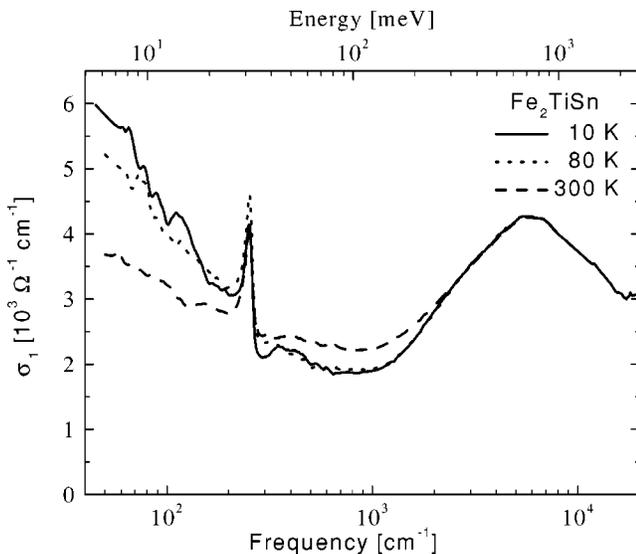
FIG. 2. The optical conductivity  $\sigma_1(\omega)$  of  $\text{Fe}_2\text{TiSn}$  is characterized by a narrow Drude mode and an interband transition at around  $7000 \text{ cm}^{-1}$ . A strong peak at  $250 \text{ cm}^{-1}$  is an optically active phonon mode.
