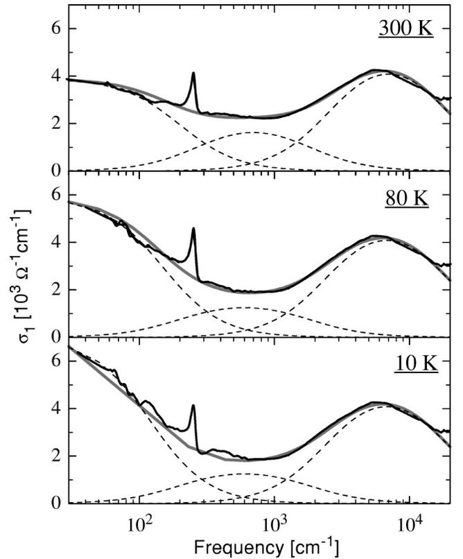
FIG. 3. Drude-Lorentz fits of the optical conductivity  $\sigma_1(\omega)$  at 300, 80, and 10 K. As temperature decreases, the Drude peak narrows, but its spectral weight appears to be conserved. The  $7000 \text{ cm}^{-1}$  peak is only weakly temperature dependent.
