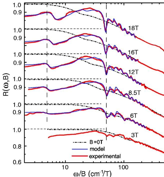
FIG. 3. (Color online) The  $\omega/B$  scaled plot of the *ab*-plane reflectance spectra  $R(\omega, B)$  in several magnetic fields. At each field  $B$ , the zero field reflectance spectrum  $R(\omega, B=0)$  is also scaled by the corresponding factor  $B$  for comparison. Every set of spectra is offset by 30% for clarity. The model spectra are obtained from the analysis detailed in the text.
