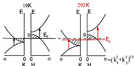
FIG. 2. (Color online) Schematics of the band structure of graphite at  $K$  and  $H$  points of the Brillouin zone at 10 and 292 K. The arrows indicate the interband transitions observed in the bottom inset of Fig. 1.
