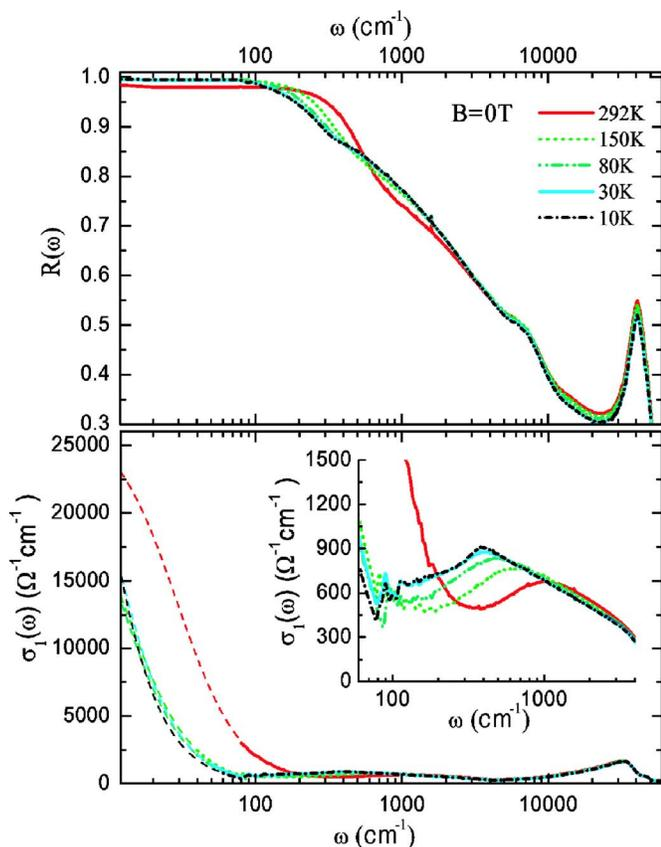
FIG. 1. (Color online) Zero field *ab*-plane reflectance  $R(\omega)$  (top panel) and real part of the optical conductivity  $\sigma_1(\omega)$  (bottom panel) of graphite. The thin dashed lines in the bottom panel are Drude fits of the  $\sigma_1(\omega)$  spectra in the low frequency region. The bottom inset displays the absorption peak of  $\sigma_1(\omega)$  in the mid-IR region, which shifts to high energy with increasing temperature.
