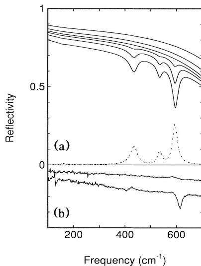
FIG. 1. (a) Theoretical  $c$ -axis loss function (dotted, arbitrary units along the vertical axis) and reflectivity (solid). From top to bottom:  $s$ -polarized light with a  $\phi$  of 45, 30, and 15 degrees relative to the surface normal. Lowest three curves:  $p$  polarized, same angles in reverse order. (b) Reflectivity of  $Tl_2Ba_2Ca_2Cu_3O_{10}$  for  $s$  (upper curve) and  $p$ -polarized light (lower curve) taken with  $\phi = 45$  degrees.
