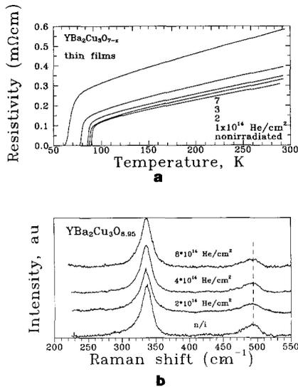
**Fig. 1.** (a) Temperature dependence of the dc resistivity of  $\text{YBa}_2\text{Cu}_3\text{O}_{7-x}$  thin films irradiated with 160-keV  $\text{He}^+$  ions. (b) Raman spectra from the  $ab$ -face of a  $\text{He}^+$  irradiated single crystal of  $\text{YBa}_2\text{Cu}_3\text{O}_{6.95}$ .
