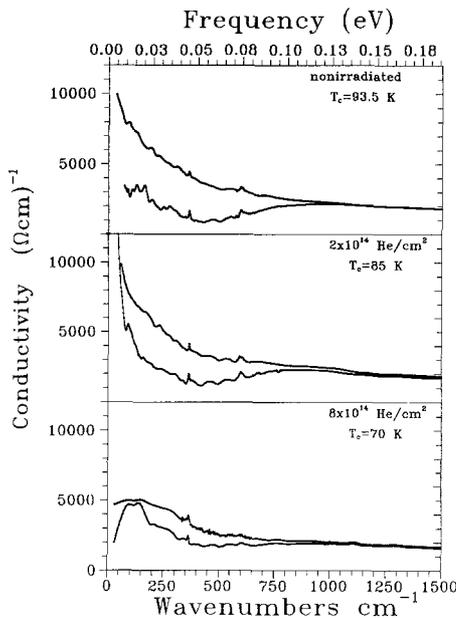
**Fig. 2.** Frequency dependence of the optical conductivity of the  $\text{He}^+$ -irradiated single crystal of  $\text{YBa}_2\text{Cu}_3\text{O}_{6.95}$ . Upper curves in all panels were obtained at a temperature slightly above  $T_c$  while bottom curves were obtained at 10 K.
